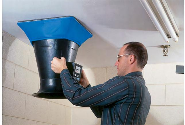
The LoFlo Balometer® Capture Hood is mainly used in residential or light commercial applications for taking measurements from 10 to 500 cfm (17 to 850 m<sup>3</sup>/h). The compact size allows them to be used where full size hoods would not fit such as over bathroom stalls or filing cabinets.
